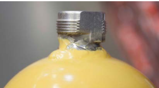
Bernzomatic/Worthington Map/Pro cylinder found on shelf at Home Depot, El Cerrito, CA, as shown, on February 12, 2012, evidences weld repair then sale as a new cylinder.
