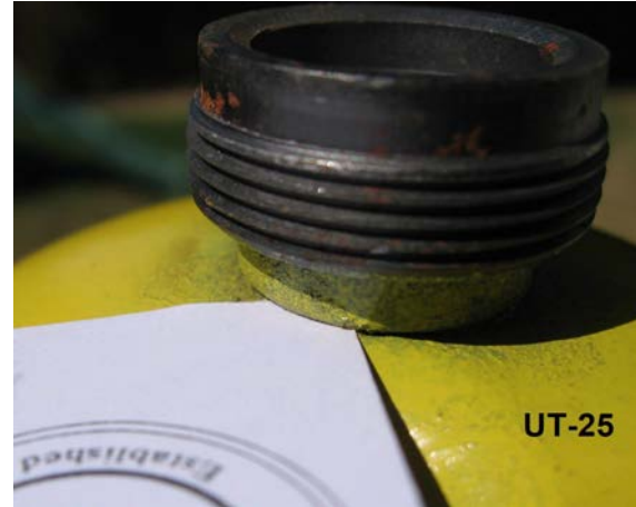
Poorly brazed joint as found on the shelf at Home Depot.
